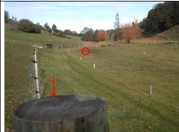
Figure S54. Frenchman's Gully, Lakes Entrance Victoria. Piezometers (made of agi-pipe) at this site have not only helped us to plan the plantings on the valley floor by mapping soils and water table depth, they have also assisted in assessing the amount of processing by the rainforest planting of phosphorus in the water table (which ultimately ends up in the Gippsland Lakes). The red arrow marks the point and the circle in Figure S53 two years later.
