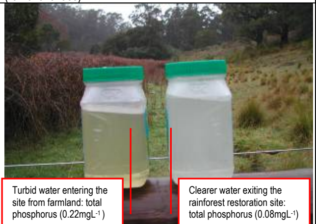
Figure S57. Frenchman's Gully, Lakes Entrance Victoria. The water shown in these two jars graphically illustrates a 70% stripping of phosphorus from the floodwaters of Maringa Creek: a 4-year-old rainforest restoration site. See the cover figure to Chapter S3 to understand the usefulness of these results in changing social attitudes towards rainforest restoration and the wider environment.
